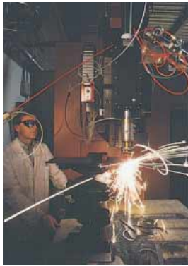
Figure P34.21 A laser cutting device mounted on a robot arm is being used to cut through a metallic plate. (Philippe Plaitly/SPL/Photo Researchers)
