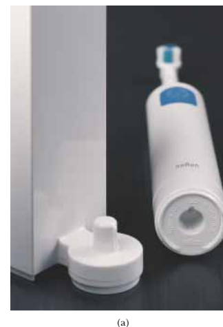
Figure 32.13 (a) This electric toothbrush uses the mutual induction of solenoids as part of its battery-charging system. (b) A coil of N_H turns wrapped around the center of a solenoid of N_B turns.
