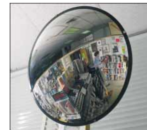
Figure 36.16 Convex mirrors, often used for security in department stores, provide wide-angle viewing.
