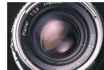
This camera lens has several coatings (of different thicknesses) that minimize reflection of light waves having wavelengths near the center of the visible spectrum. As a result, the little light that is reflected by the lens has a greater proportion of the far ends of the spectrum and appears reddish-violet.
