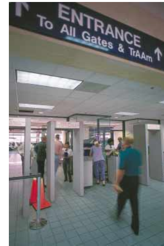
Figure 33.17 When you pass through a metal detector, you become part of a resonant circuit. As you step through the detector, the inductance of the circuit changes, and thus the current in the circuit changes. (Terry Qing/IFPG International)
