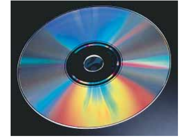
Figure 38.22 A compact disc observed under white light. The colors observed in the reflected light and their intensities depend on the orientation of the disc relative to the eye and relative to the light source.
