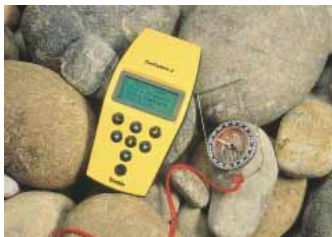
This Global Positioning System (GPS) unit incorporates relativistically corrected time calculations in its analysis of signals it receives from orbiting satellites. These corrections allow the unit to determine its position on the Earth's surface to within a few meters. If the corrections were not made, the location error would be about 1 km. (Courtesy of Trimble Navigation Limited)
