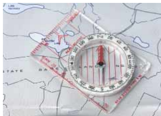
The north end of a compass needle points to the south magnetic pole of the Earth. The "north" compass direction varies from true geographic north depending on the magnetic declination at that point on the Earth's surface.
