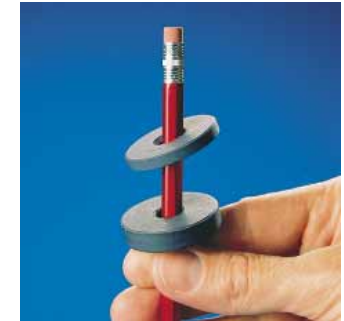
Figure Q30.33 Magnetic levitation using two ceramic magnets.
