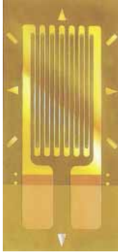
The strain gauge, a device used for experimental stress analysis, consists of a thin coiled wire bonded to a flexible plastic backing. The gauge measures stresses by detecting changes in the resistance of the coil as the strip bends. Resistance measurements are made with this device as one element of a Wheatstone bridge. Strain gauges are commonly used in modern electronic balances to measure the masses of objects.
