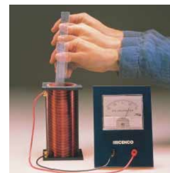
Figure 31.14 When a magnet is moved toward or away from a solenoid attached to a galvanometer, an electric current is induced, indicated by the momentary deflection of the galvanometer needle. (Richard Megna/Fundamental Photographs)
