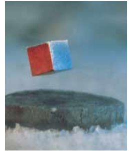
A small permanent magnet levitated above a disk of the superconductor \text{YBa}_2\text{Cu}_3\text{O}_7 , which is at 77 K.
