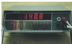
Figure 28.26 Voltages, currents, and resistances are frequently measured with digital multimeters like this one.
