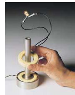
A demonstration of electromagnetic induction. A changing potential difference is applied to the lower coil. An emf is induced in the upper coil as indicated by the illuminated lamp. What happens to the lamp's intensity as the upper coil is moved over the vertical tube? (Courtesy of Central Scientific Company)
