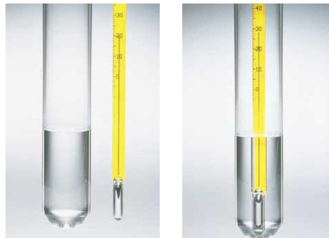
Figure 19.1 As a result of thermal expansion, the level of the mercury in the thermometer rises as the mercury is heated by water in the test tube.
