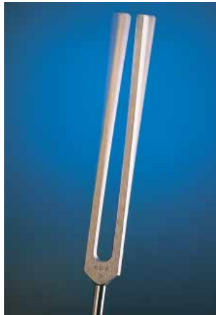
The sound from a tuning fork is produced by the vibrations of each of its prongs.
