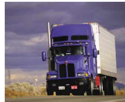
The high cost of fuel has prompted many truck owners to install wind deflectors on their cabs to reduce drag.
